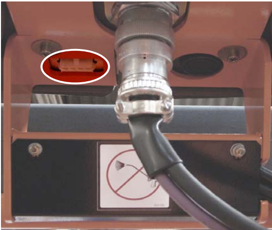
Figure 9-2. Hand Held Analyzer Connection
