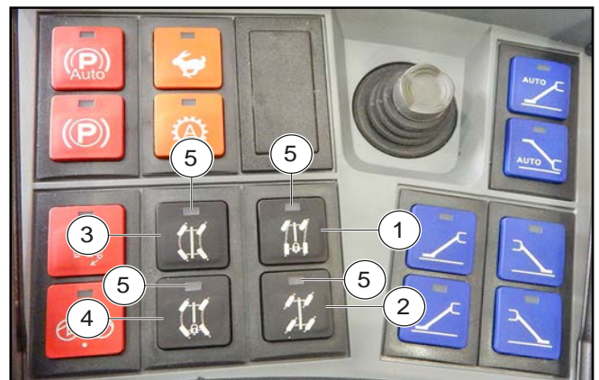
Figure 128: Mode de direction
