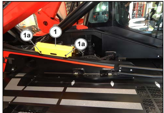
Figure 210: Boom safety wedge
