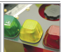
Overload warning lamps + auto stop + alarm
